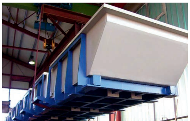
Pickling plant in PP
